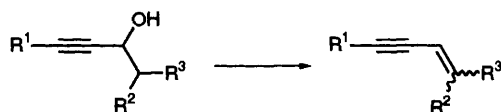
Scheme 1 Reagents and conditions: substrate (1 mmol), PdCl 2 (PPh 3 ) 2 (10 mol%), SnCl 2 (1.5 mmol), DMI (1.5 ml), 70 °C
